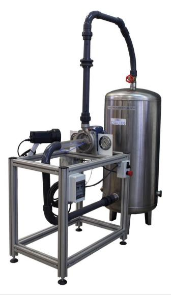
Cavitation is produced when a liquid that is being pumped loses pressure and matches the level at which vapour is generated at the same temperature the pump is operated. At that moment, liquid turns into vapour, giving rise to vapour locks or vacuum pockets that are pushed into other areas with a higher pressure. Very fast condensation takes place creating short-lived excess of pressure in very small places.
